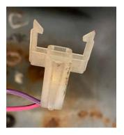
21. Remove the spring clip retaining the brake master cylinder pushrod – a small hook tip tool works well, or needle nose pliers. Note that the pushrod has more
