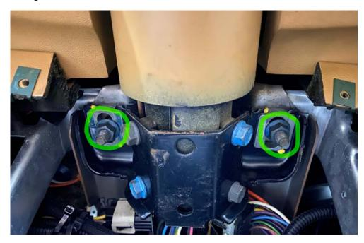
7. Now it's time to explore the many wiring harnesses that attach to your steering column. Each one surprises with its own release tab location.
