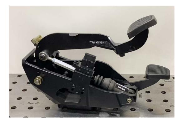
c. The clutch pedal stop screw is pre-installed at the approximate right height. Ensure the nut is tight against the pedal arm. This can be adjusted at a later point if needed.
