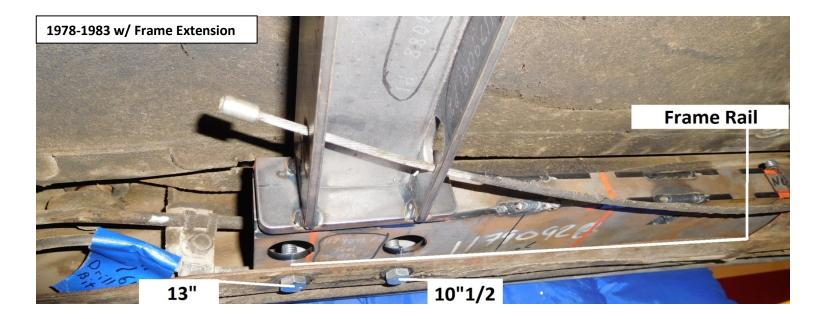
2. Carefully raise up the rear tail shaft of the transmission to slide in the cross-member and secure to the frame rail or the frame extensions if used. Once bolted in, install the supplied transmission mount to cross-member and the transmission.
