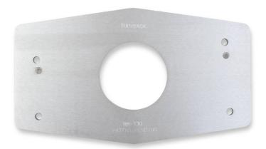
Congratulations on your purchase of the QuickTime RM-130 Index Plate. The RM-130 Index plate is used when indexing (centering) any QuickTime T56 bellhousing or any OE T56 Bellhousing onto an engine.
