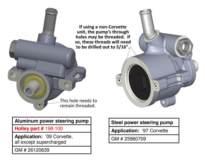
The Holley driver's side bracket uses the standard (1997 and up) Corvette power steering pump (Saginaw TC type). Other pumps of the same housing and type may work, but the bracket is optimized for the Corvette pump.
