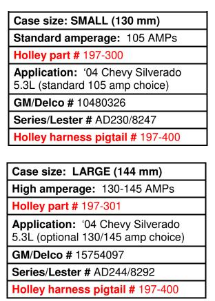
The Holley driver's side bracket uses standard alternators with 5.46" bolt spacing. This alternator type is common on most '96-'05 GM trucks and '98-'06 Camaro/Firebird/GTOs. There are two alternator amperages available in this type. Note: The Holley bracket DOES NOT work with '97-UP Corvette or '10-UP Camaro alternators which have 6" (154 mm) center bolt spacing.
