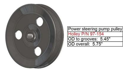
WARNING! Smaller power steering pulleys, such as a 97-154 can rotate the pump beyond recommended RPMs. To correct this, a 25% under-dive balancer should be used if choosing a pump pulley smaller than 6" OD.
