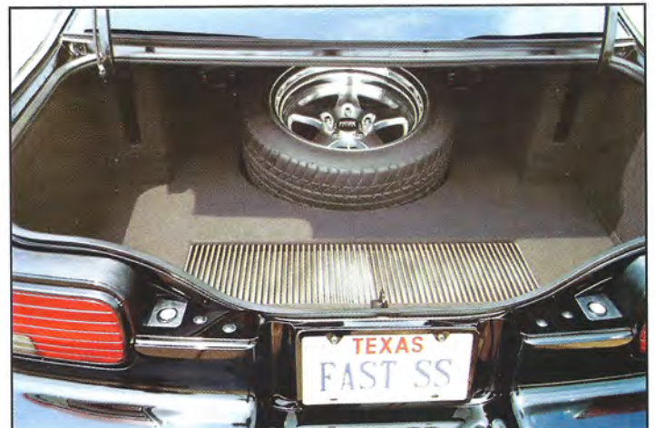
Look closely and you may catch a glimpse of the sub-woofers, on either side of the spare tire. The amps, the wiring and all the rest of the stereo installation are tucked away in one of the cleanest installs you'll find!
