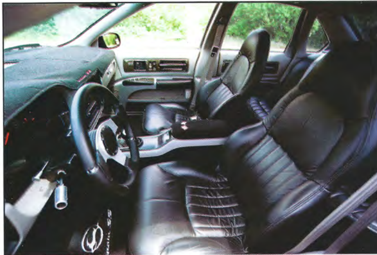
Sweet, sweet black and gray interior featuring C5 Corvette seats, six speed transmission, Momo steering wheel and Momo shift knob, Z28 instrument cluster, carbon fiber and billet trim. Yeah, that'll do!
